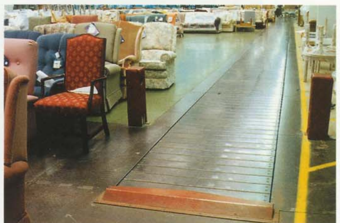
6. IN FLOOR CONVEYORS
