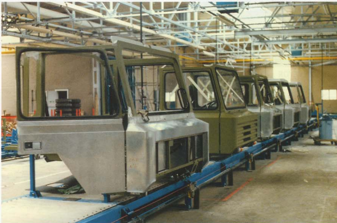
2. CAB ASSEMBLY CONVEYOR
