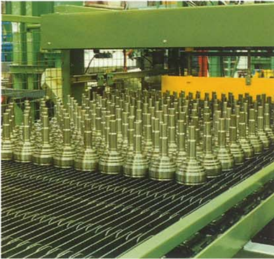
1. HEAT TREATMENT CONVEYOR
